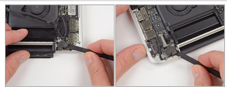
• Use the flat end of a spudger to pry the rubber hinge covers up off the left and right hinges.
